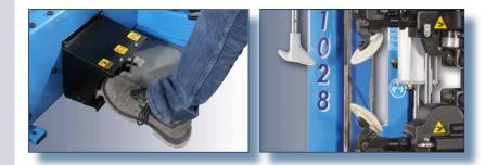
Manual rotation allows the operator to switch between demounting and mounting mode quickly and easily.
